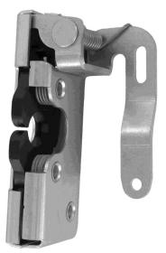
This two rotor latch is a sub-platform to the Tri*Mark* proven 050-0100 series latch and is designed for medium to heavy-duty applications for on or off highway entrance doors, compartments and access panels. It features a coaxial trip mechanism for applications where it is desirable to provide additional support to the trip lever and is FMVSS 206 compliant.
